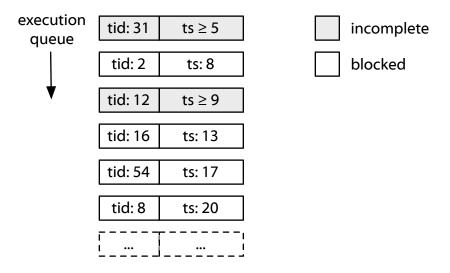
Figure 5.3: Queue of logged transactions at a stalled repository, in timestamp order. The shaded transactions are *incomplete* awaiting votes from a failed participant and do not yet have a final timestamp. The non-shaded transactions have a final timestamp, but are *blocked* behind incomplete transactions, waiting to be executed in timestamp order.
