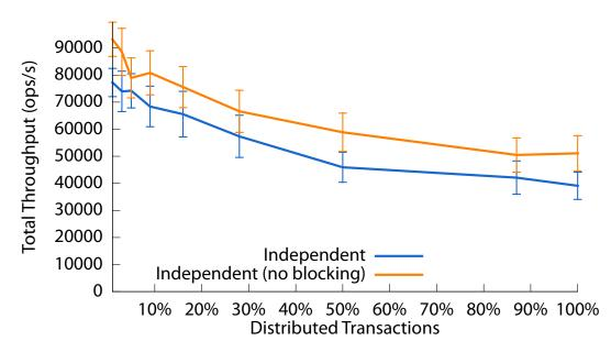
Figure 6.8: Two-repository throughput in *operations* per second, with an increasing proportion of distributed transactions. We examine topologies where the two repositories are located on the same LAN, and when they are separated by a 10 ms one-way network delay.
