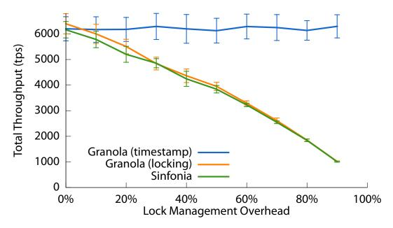
Figure 6.9: Two-repository throughput for a workload comprised of 100% distributed transactions with no lock contention, as a function of cost of managing locks. The cost of locking is expressed as a fraction of total CPU time to execute the transaction. We examine Granola in both timestamp mode and locking mode, as compared to the Sinfonia protocol.
