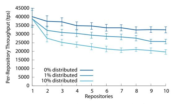
Figure 6.7: Per-repository throughput with a varying number of total repositories, for workloads comprised of a varying fraction of independent transactions. Each distributed transaction is issued to two repositories, with a single master.
