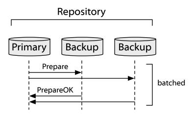
Figure 5.1: The basic Viewstamped Replication protocol as used in Granola to provide stable log writes. More complex communication is required when issuing a view change to recover from node failures.
