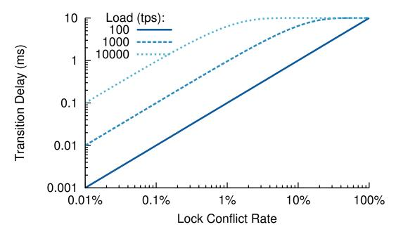
Figure 6.11: Expected delay when transitioning to locking mode ( $D_{coord}$ ), for a given lock conflict rate ( $C_{ind}$ ) and independent transaction load ( $\lambda_{ind}$ ). Transaction processing time ( $W_{ind}$ ) is set to 10 ms.
