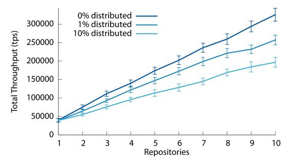
Figure 6.6: Total system throughput with a varying number of repositories, for workloads comprised of a varying fraction of independent transactions. Each distributed transaction is issued to two repositories, with a single master.
