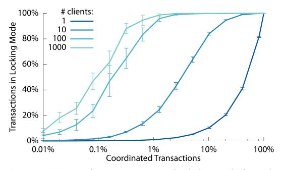
Figure 6.14: Fraction of transactions processed in locking mode, for workloads composed of a varying fraction coordinated transactions. We examine a varying number of concurrent client connections. 100 clients are sufficient to fully-load the repositories in this benchmark.
