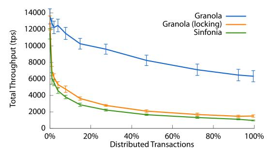
Figure 6.17: Two-repository throughput on a version of the TPC-C benchmark that issues only new\_order requests, with a variable rate of distributed transactions. We examine both the Granola and Sinfonia protocols, along with a version of Granola that uses only coordinated transactions.
