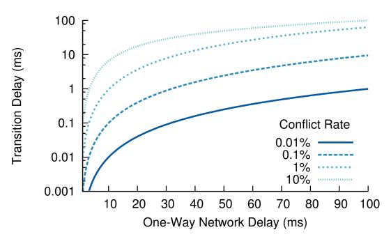
Figure 6.12: Expected delay when transitioning to locking mode ( $D_{coord}$ ), for a given lock conflict rate ( $C_{ind}$ ). The one-way network delay between transaction participants approximates the time an independent transaction is active at each repository ( $W_{ind}$ ). Independent transaction load ( $\lambda_{ind}$ ) is set at 1,000 tps.
