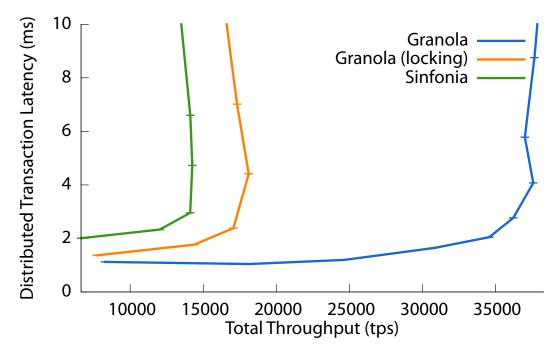
Figure 6.18: Latency for distributed transactions as a function of system throughput, showing congestion collapse for Granola, Granola in locking mode, and Sinfonia, on a six-node topology running the TPC-C benchmark.
