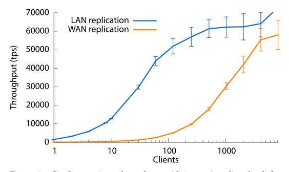
Figure 6.2: Single-repository throughput with increasing client load, for both local-area and wide-area replication configurations.
