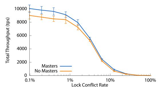
Figure C.4: The impact on throughput by avoiding transaction aborts in a master-based protocol, for a bifurcated network topology with workload comprised of 100% coordinated transactions on two repositories. The repositories are separated by 10 ms one-way bifurcation delay, and half the clients are colocated with each repository. The master is located mid-way between the two repositories.
