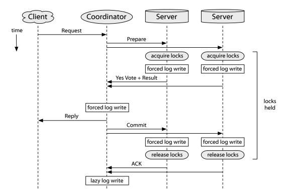
Figure 2.1: Traditional two-phase commit protocol, as applied to a oneround transaction model. Locks must be acquired for the duration of the transaction, and multiple forced log writes must be written on both the participants and the coordinator.
