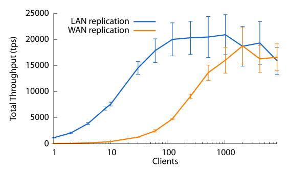
Figure 6.4: Total throughput with increasing client load for a two-repository system with 100% independent transactions, for both local-area and wide-area replication configurations.
