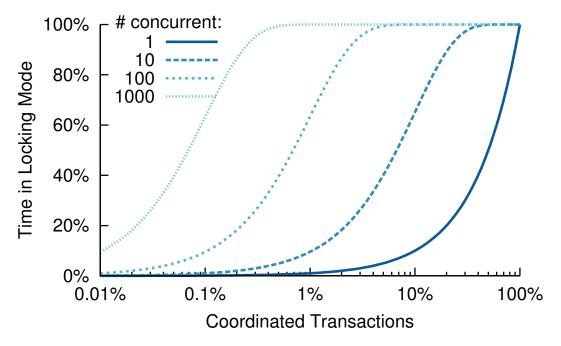
Figure 6.13: Expected time spent in locking mode at a repository ( $T_{coord}$ ), as a function of the fraction of coordinated transactions ( $P_{coord}$ ) and number of concurrent distributed transactions ( $L_{dist}$ ).
