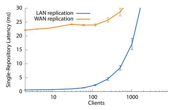
Figure 6.3: Per-transaction latency for single-repository transactions, with increasing client load, for both local-area and wide-area replication configurations.
