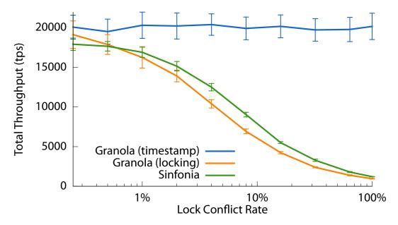
Figure 6.10: Two-repository throughput for a workload comprised of 100% distributed transactions, as a function of the lock contention rate. We examine Granola in both timestamp mode and locking mode, as compared to the Sinfonia protocol.
