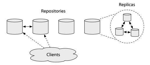
Figure 3.1: Granola system topology. This figure shows the clients and repositories, as well as the individual replicas that make up each repository.
