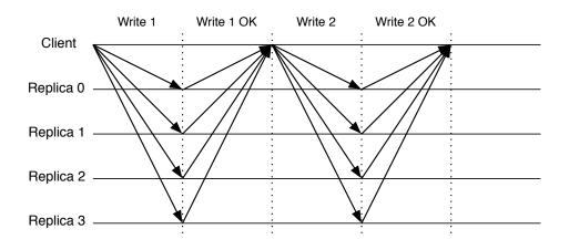
Figure 3-1: HQ Normal-case Communication
